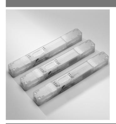
The DA-SL-AD series are a range of DALI addressers that can be setup using simple to use DIL switches. An addresser takes in a message from an addressable DALI system and translates it into a broadcast message so that the luminaire ballast(s) does not have to be addressed using a PC or other methods.
